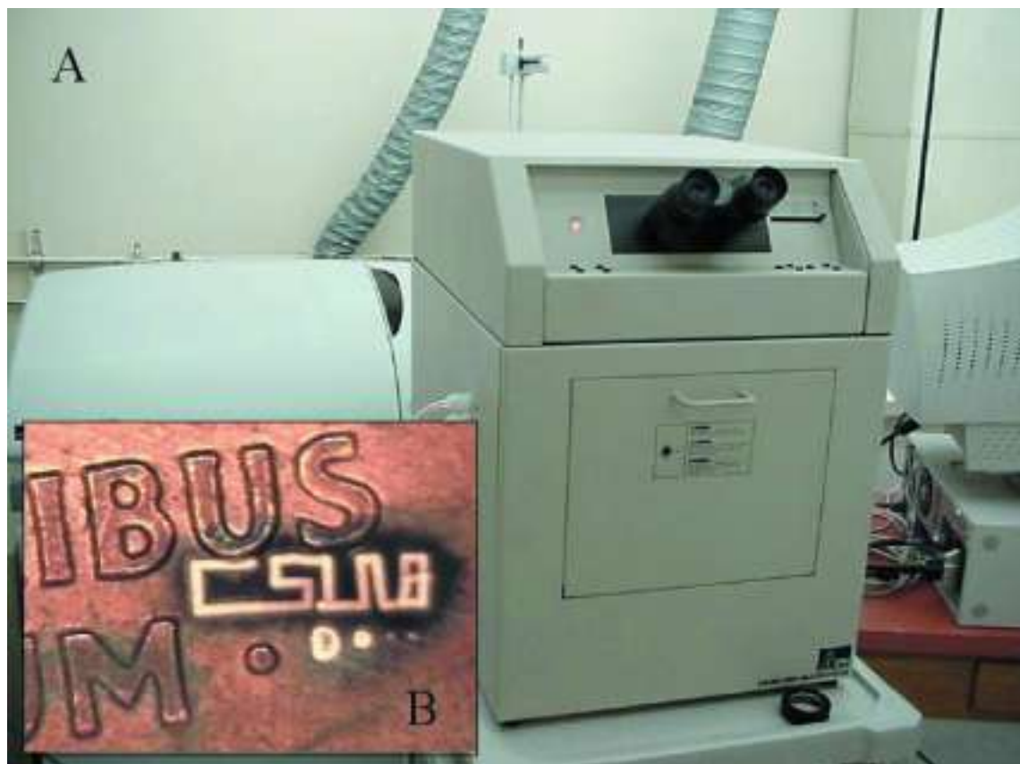
Figure 4a. Cetac Laser ablation system at CSULB; 4b (inset). CSULB ablated under E-PLURIBUS on the back side of a penny.
