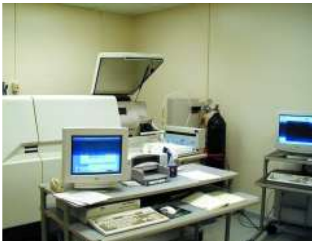
Figure 2. VG Axiom magnetic sector ICP-MS recently installed at MURR.
